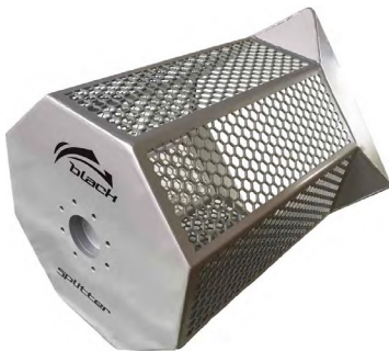
SCREENING BASKET 40mm grid, produces 30mm downwards material. Four flat edges for easy loading and flat sides create efficient tumbling / screening action
